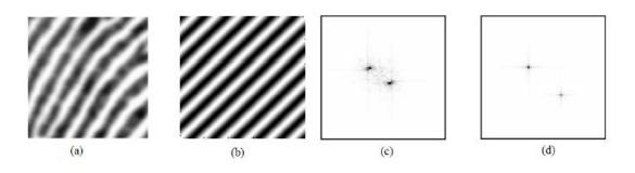
Figure 2.8: Surface wave approximation: (a) Local region in a fingerprint image (b) Surface wave approximation (c,d) Fourier spectrum of the real fingerprint and the surface wave. The symmetric nature of the Fourier spectrum arrives from the properties of the Fourier transform for real signals
